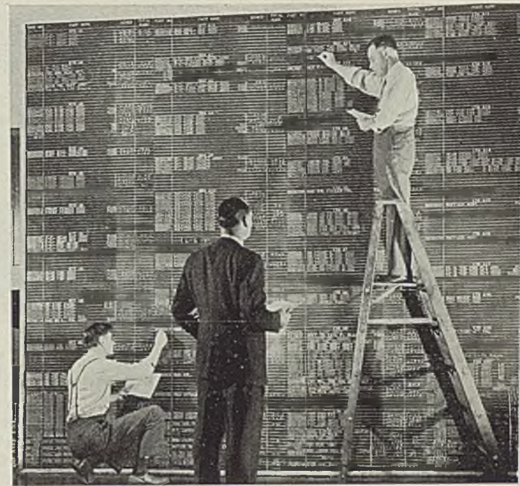
■ Not the least of many factors in automotive productive ingenuity is the ability to schedule parts to arrive at assembly lines simultaneously and in adequate quantities. Assembly, key operation of production, could not go on were even the smallest part not ready at the appointed time and place. Here, at a huge control board Chevrolet superintendents balance and control flow of parts
