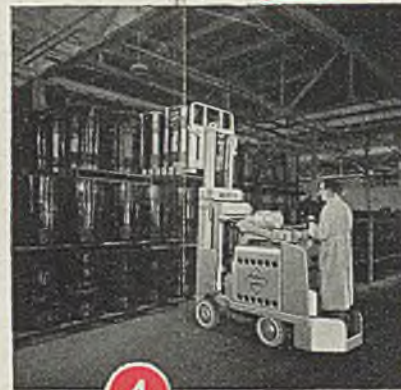
Triple-Lift Electric Fork Truck lifts loads up to 112" — or to roof girders.
