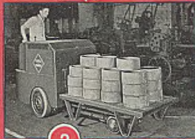
Electric Platform Truck delivers skid loads to machines.
