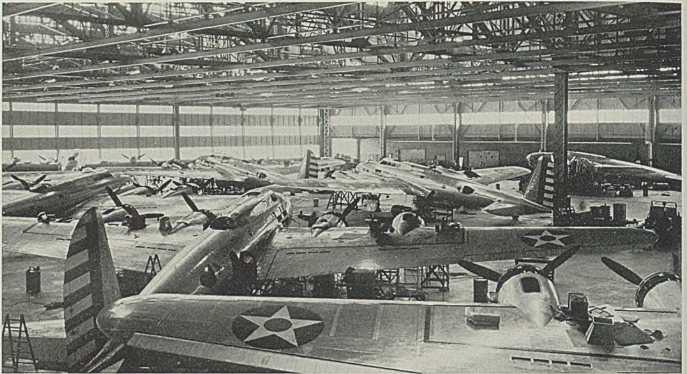
Fig. 4—Monorail bridges also serve final assembly area in new 300-foot bay at Boeing plant No. 2. Note how small men appear working on plane in extreme right, rear, just to right of pillar
