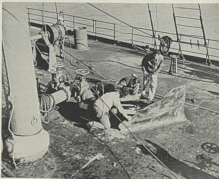
■ Survivors of the S. S. MALAY, United States tanker damaged by an Axis torpedo off the Atlantic coast, examine the ripped deck plates after the ship limped into Newport News, Va. NEA photo
