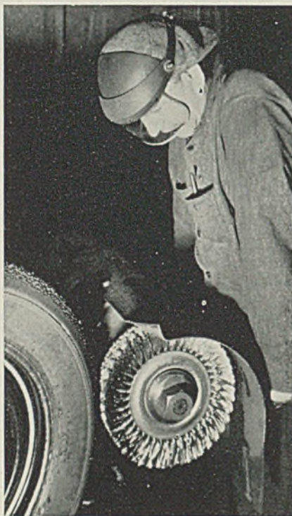
A brush for recapping and retreading tires has been developed by Osborn Mfg. Co., Cleveland. Strands are "rope twisted" with needlepoint wires. It is claimed the construction "prevents shedding, flaring or spreading of the brush, and every wire point is brought into action." The purpose is to furrow a tire's surface closely, for better adhesion of rubber applied to it
