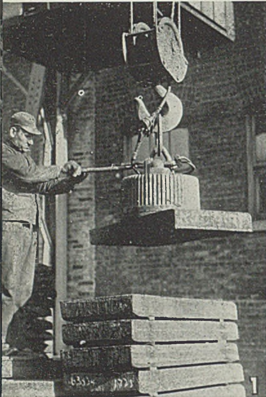
Fig. 1—Circular magnet for handling slabs and plates
