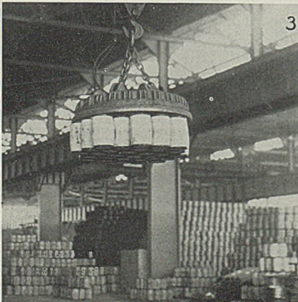
Fig. 4—Two coils weighing 56,600 pounds being lifted by magnet of coil type
