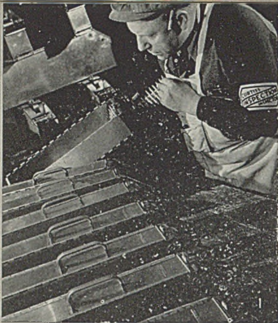
Fig. 1—Here an inspector checks feed of cartridge belt from ammunition box by inserting cartridges and withdrawing them. Note how top of box is secured by double hinge and through pins
