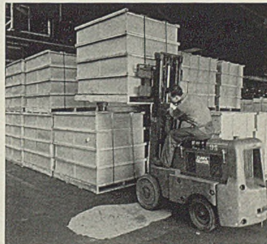
Fig. 3—Swift unloading and storage at recipient's plant also is done with fork type lift trucks. Tying two and three high utilizes storage areas with maximum efficiency
