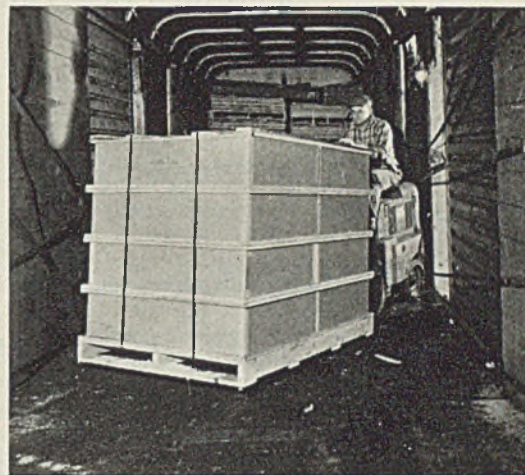
Fig. 2—A gasoline-powered fork lift truck loads the unit packages into the freight car at the vendor's plant in minimum time and at low cost
