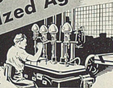
Drilling, tapping or reaming aircraft engine main bearing liners at Ampco.
