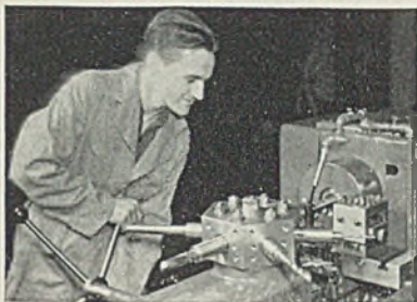
Oster No. 601 equipped with six position turret having six tapped holes in each face for mounting a wide variety of tool holders.
