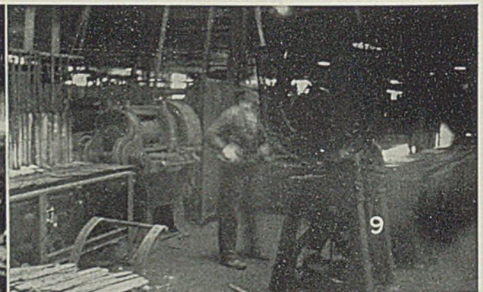
Fig. 10—After eye is rolled up on one end of the volute spring blank, entire blank is heated in this big chain conveyor furnace preparatory to forming
