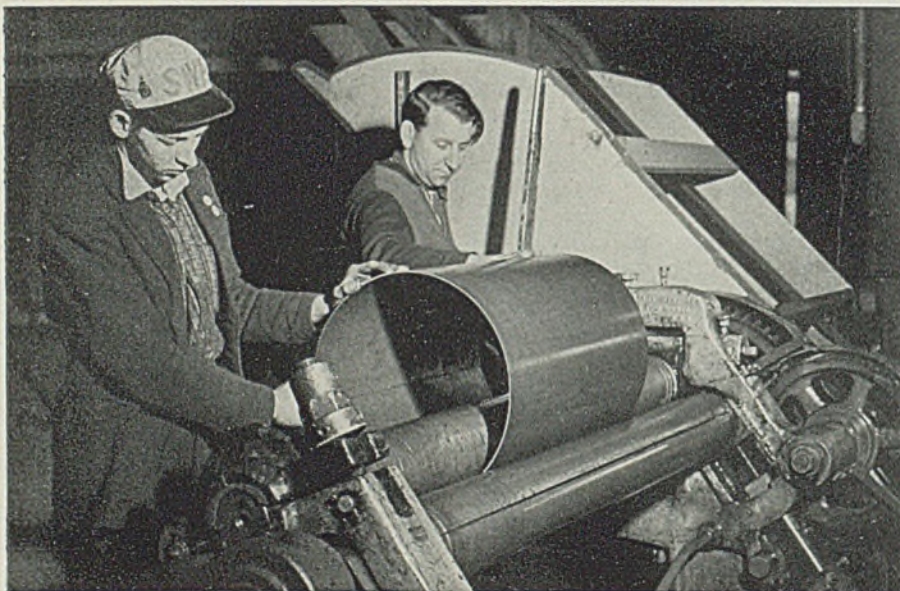
CANADIAN war factories are speeding up production of depth charges to intensify the battle against raiding Axis submarines. Here workers force steel plates through bending rolls to form the sides of the receptacles, which are filled with high explosives. NEA photo, passed by Canadian censor
