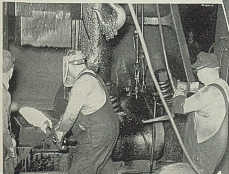
Fig. 4—Huge steam hammer exerts a pressure of 320,000 pounds per square inch. In the first of two operations on Buick crankshafts, it is used to form cheeks in one section of the dies; then in the finish impression die section, the shape is further developed. Operator at right employs air gun to keep dies clean by blowing out dirt and scale. Center man manipulates stock under the hammer. Workman at right operates the hammer controls. Portion of high-powered blower can be seen at lower left. It helps dissipate heat from work by blasting cooler air into the working zone.
