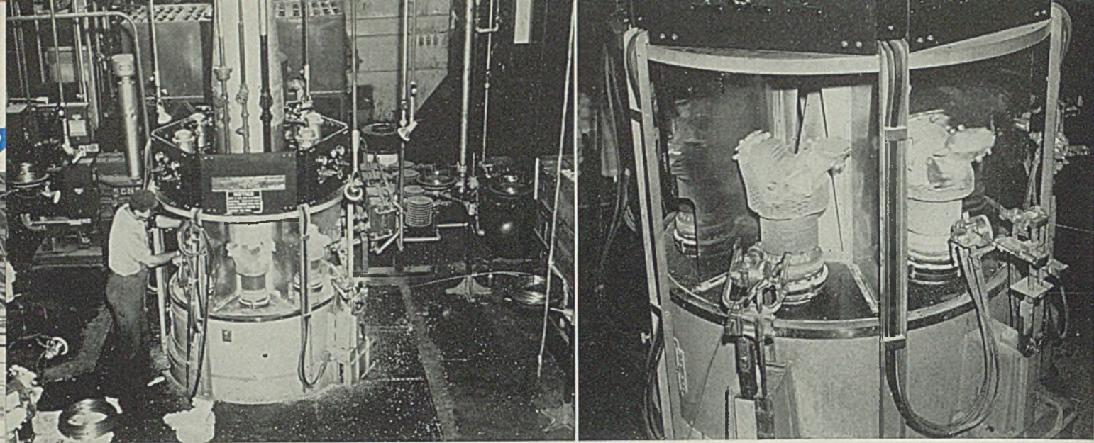
Fig. 1—(Left, above)—General view of automatic metal spraying layout. Left rear, air compressor; right rear, air drier; center, 6-station automatic metallizing machine. Note gages and controls mounted above each of the 5 operating stations. The sixth, in front here, is the loading-unloading station
