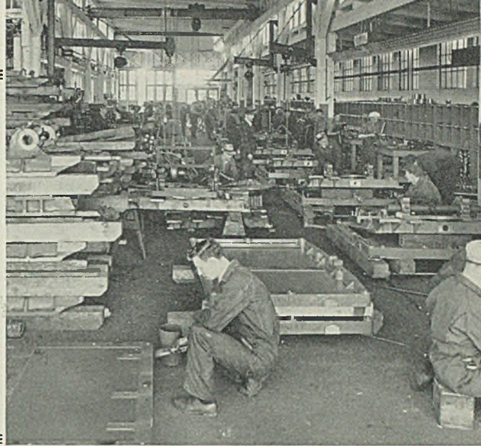
Fig. 1—Above, view of the steam steering engine assembly line as seen from the starting end
