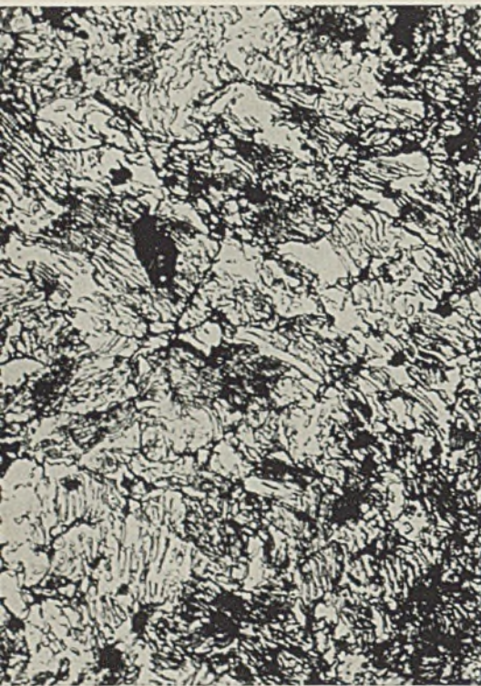
Fig. 3. (Left)—Micrograph of powdered metal compact exhibits alternate layers of iron and carbides, the light areas being the iron; the dark, the carbides. Black patches are pores which contain some free graphite
