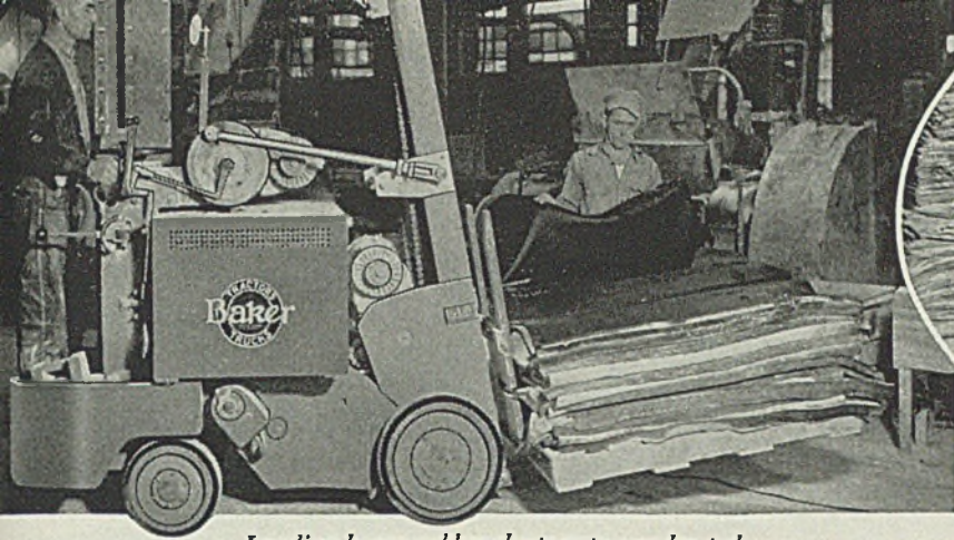
Loading heavy rubber sheets onto wooden pallets, carried by Baker 2000 lb. Fork Truck.
