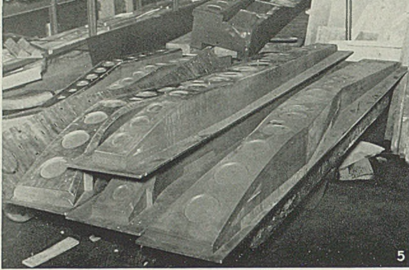
Fig. 5—Dies made from vulcanized fiber, some of them 6 feet long, are mounted on steel backing plates and used successfully in forming by the Guerin process. Formed stampings are seen over two of the dies here. At the left is a templet used in making one of the dies
