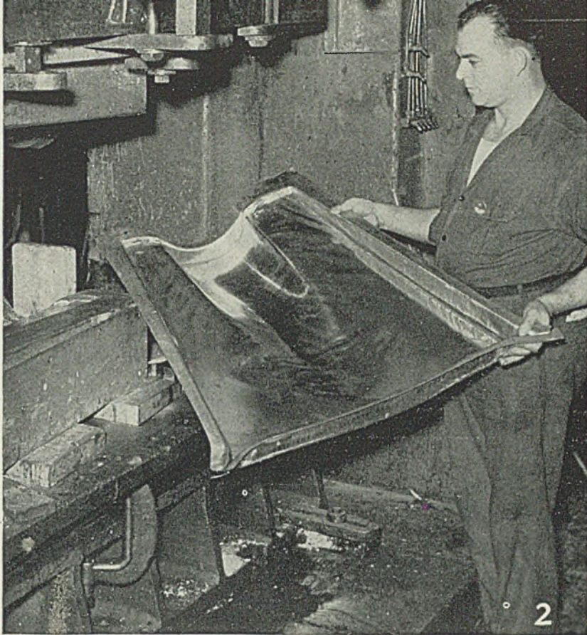
Fig. 1—One of many zinc alloy dies (Kirk-site) now being used successfully for deep drawing aircraft parts in double-acting crank presses is shown here. Both die and punch as well as pressure ring are cast close to finished dimensions
