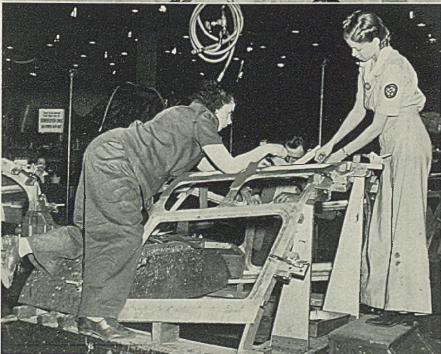
WOMEN have a major role in the production of heavy bombers at Consolidated Aircraft Corp.'s large plant at San Diego, Calif. Famed B-24s now are being produced on a continuously moving assembly line (see STEEL, March 23, p. 31). Upper photo, women workers are operating drills on stampings in parts department. Lower photo, two women and a man assemble part of the nose for a B-24.
