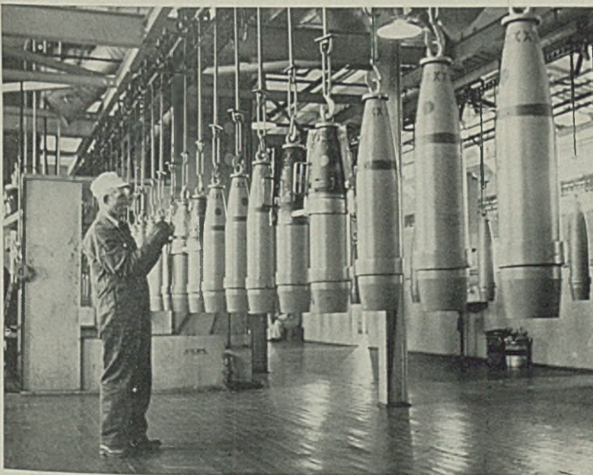
SLOWLY revolving on an overhead conveyor, these heavy shells pass through the painting room in a Canadian munition factory. A worker sprays on a protective coating with an air-pressure gun and the shells proceed to the next operation. Canadian Public Information photo, from NEA
