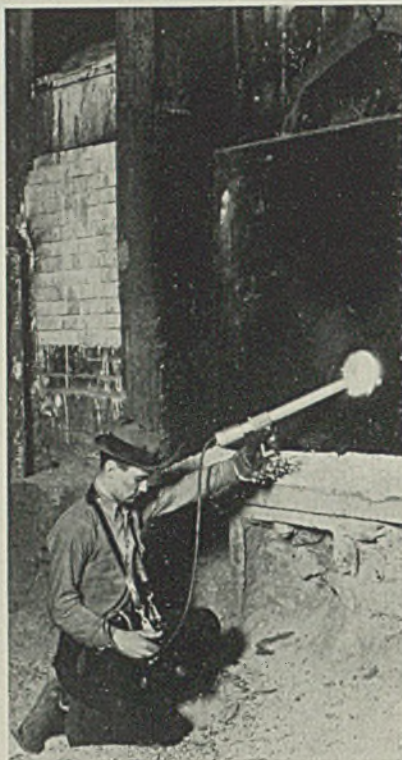
Determining temperature of a "heat" by an optical pyrometer
