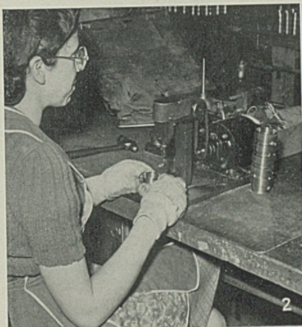
Fig. 2—The same type of burr that a dentist uses so effectively to clean cavities in teeth is employed here in a home-made machine that burrs holes on the inside of the shell boosters. Instead of waiting months for a special machine to clear up the production bottleneck at this point, the plant engineers conceived and constructed this unit in only 30 hours. That's the way brains break bottlenecks
