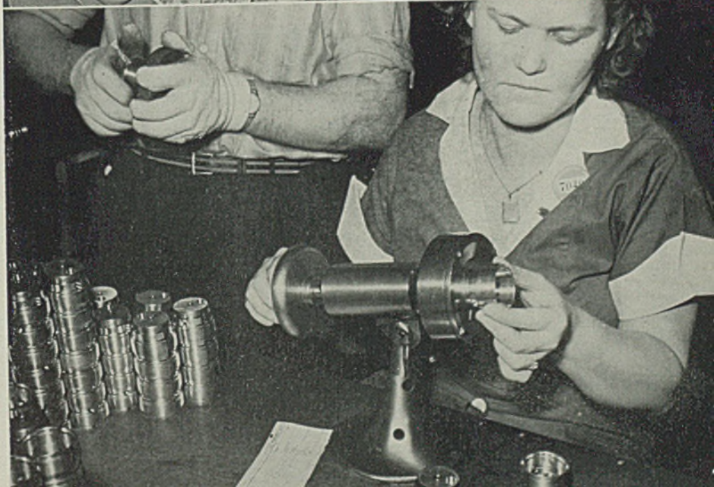
Fig. 4—Another bottleneck broken by brainwork. To save time in getting into production and permit faster operation, a plant superintendent built this machine which makes possible speedy checking of thread accuracy in contrast to older hand methods. The inventor made the machine out of a base from an electric fan and some pieces of machine steel—and in hours instead of the months that would have elapsed before such a machine could have been purchased on the open market
