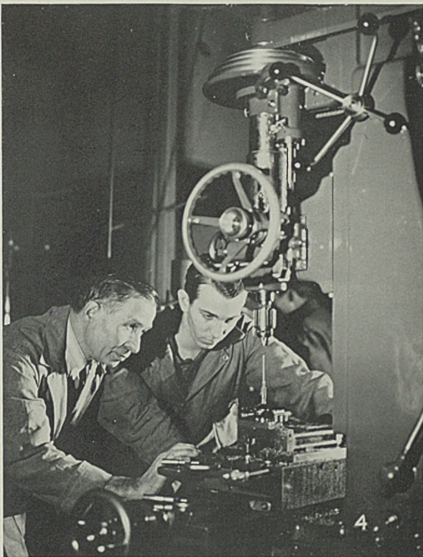
Fig. 4—Old hands and young hands—hands that used to guide machines in the manufacture of automatic vending machines—operate the same machines in the same shop, but now they make weapons for our fighting men. Here workmen are running a jig boring machine to produce a bullet die
