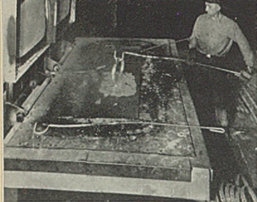
Electrically - heated galvanizing pot. Covers at left are used when bath is idle. (Courtesy Westinghouse Electric & Mfg. Co., East Pittsburgh, Pa.)
