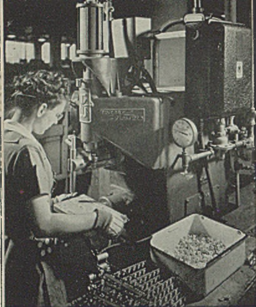
Fig. 2—Nickel plated heating racks for electric roasters are assembled in this special fixture and 29 welds are made on each unit in just one minute. About 150 completed racks are produced per hour on this setup
