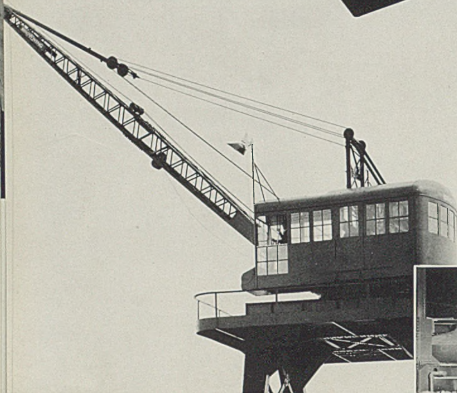
25-Ton Portal Cranes completely equipped with EC&M LINE-ARC Contactor, Time-Current Control and Type WB Brakes.
