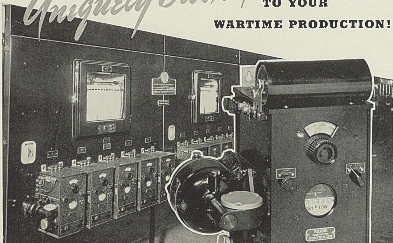
Groups of Foxboro Potentiometer Controllers like these need only one motor per group. Where records are required, a single multi-pen Foxboro Potentiometer Recorder serves each group!
