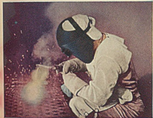
Experienced operators demonstrate the basic principles of shielded-arc welding. The use of movies makes it possible for all students in a large class to see these demonstrations close-up.
