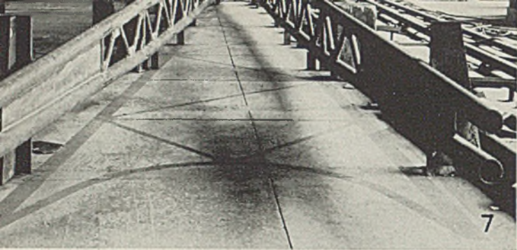
Fig. 7—Here are two completed vertical members set up ready for welding in the horizontal members. Note the markings on the floor which guide the fit-up crew in placing each tube correctly. Tubes are slotted for gusset plates
