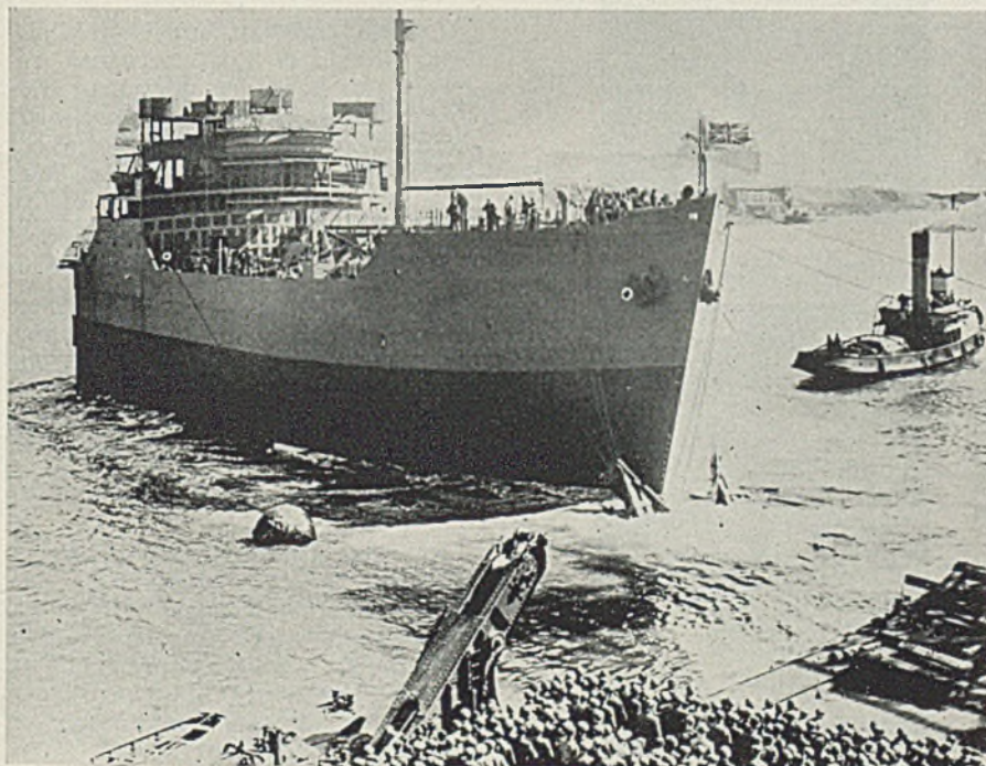
WHEN a 12,000-ton tanker struck a mine near England, the vessel broke in two and the forepart sank. The afterpart was towed into port and a new forepart built. Above photo shows the launching of the new forepart, which later was joined to the undamaged afterpart of the original tanker. The operation saved about 1500 tons of steel and the ship was rehabilitated in one-third the time that would have been required to build a new vessel. NEA photo
