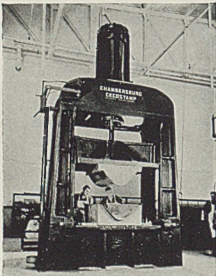
PROPELLER SPINNER. Made of stainless steel on a 66" x 48" CECOSTAMP. Rubber rings used extensively for the deep draw.
