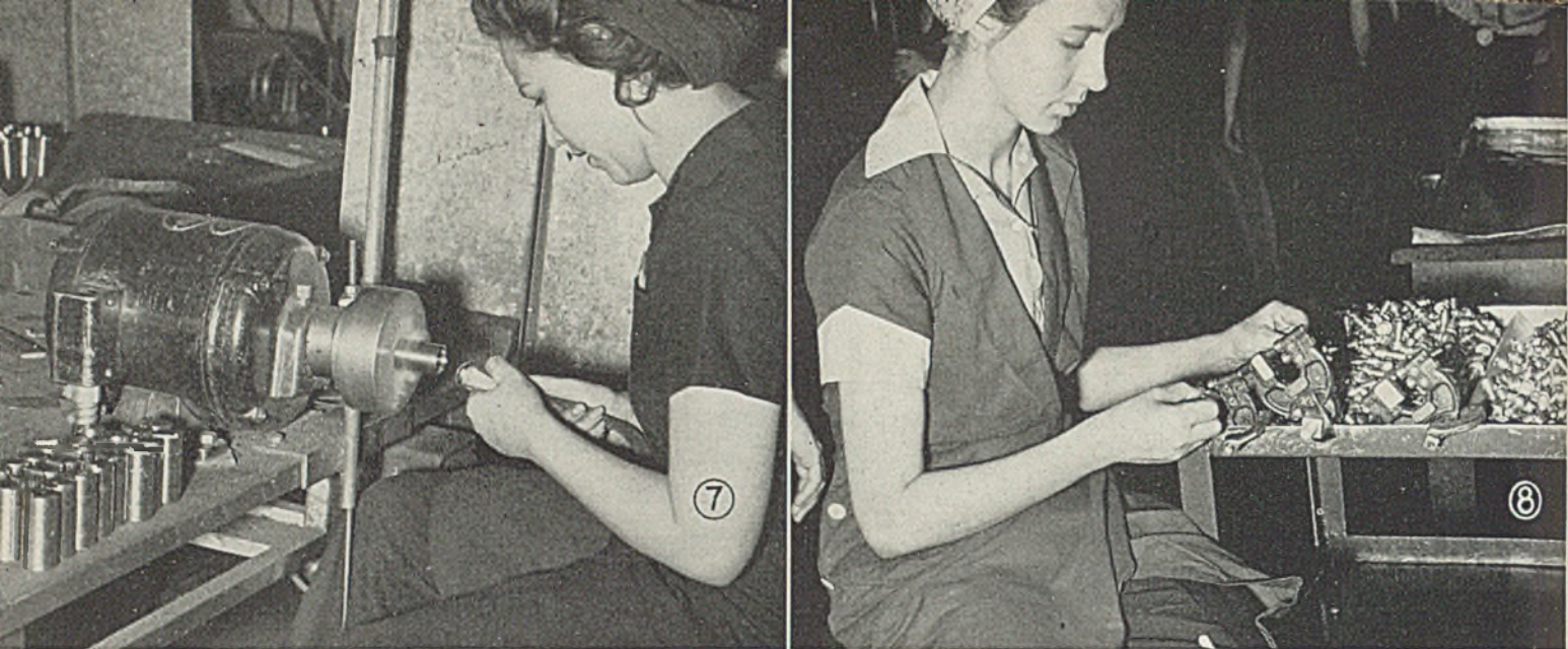
Fig. 7—Women workers are found to be particularly well fitted to handle tasks like this high-speed polishing operation. The work is held in a revolving chuck while the operator applies a strip of abrasive cloth held over a mandrel. Good touch and clear eyesight are required
