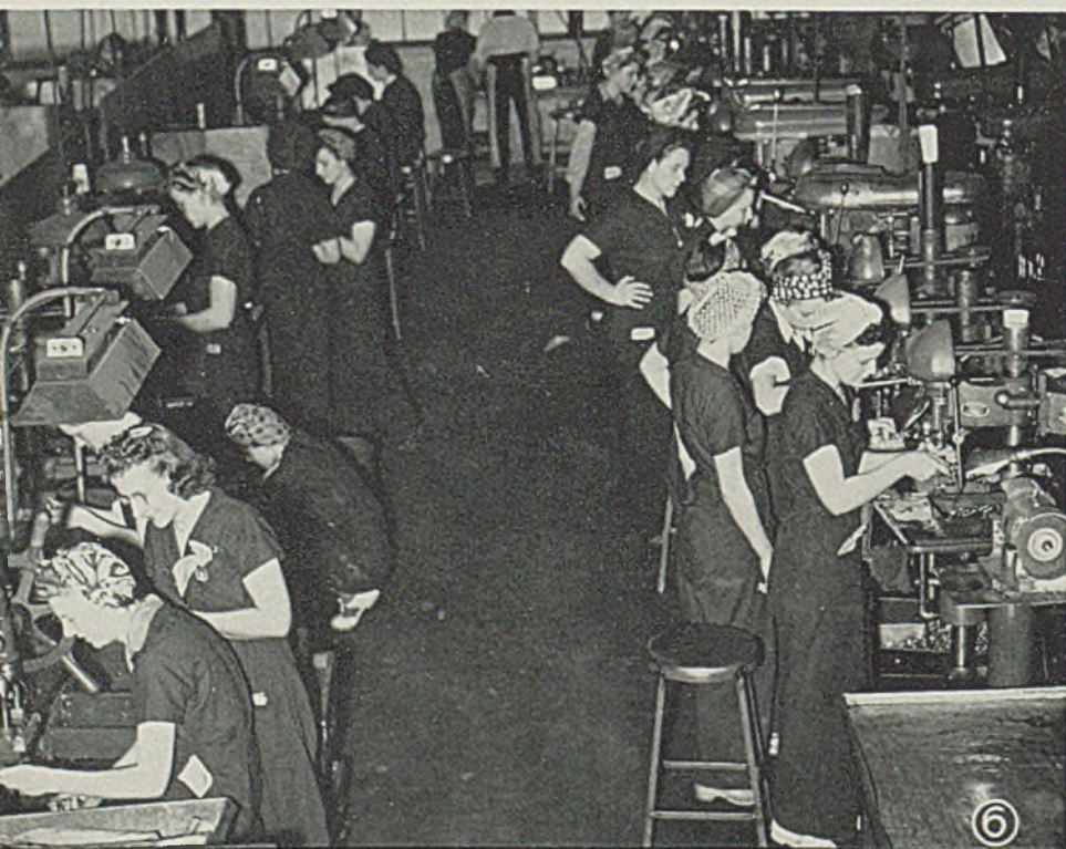
Fig. 6—WOMEN PRODUCTION WORKERS: In addition to handling practically all inspection operations, many women are employed in production work. This view shows a portion of the department devoted to machining small parts. Here experienced operators are shown instructing "trainees", standing back of them and helping them in actual production work—no artificial learning exercises, they learn to do the production operation right on the machine they will run
