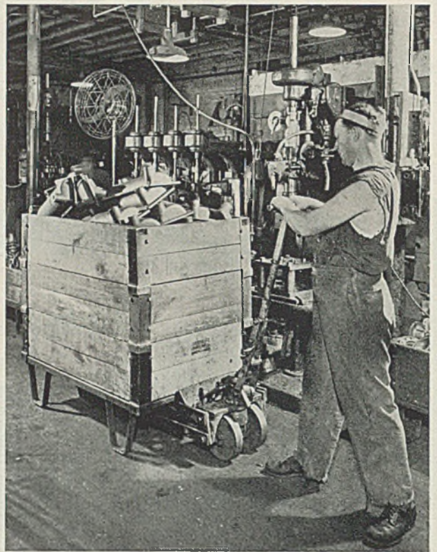
Fig. 1. (Left)—Steel strip is being moved on long skid platform by a lift-truck. Note angle iron reinforced lengthwise edge of platform and three supporting U-shaped steel legs. Fig. 2. (Right)—Reinforced wooden frames interlocked by angle irons bolted to the corners transform the skid platform into a skid box suitable for carrying parts. Note flanged angle irons which overlap frame below or platform itself
