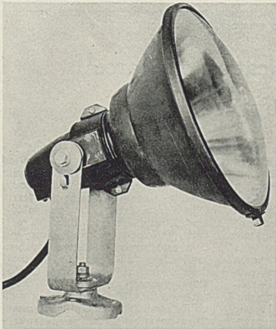
DESIGNED to eliminate vital materials needed for the war effort, General Electric Co. has developed (at left) a shatterproof floodlight entirely of glass. Reflector is coated with an electrolytically deposited metal which with an overall backing of porcelain enamel will keep the glass from shattering
