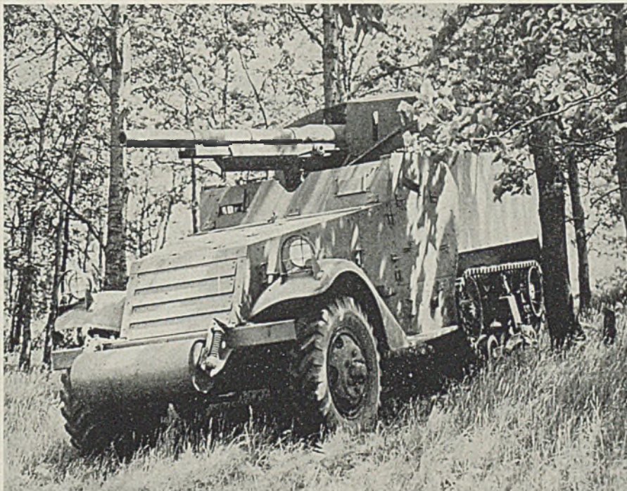
ONE of the United States' newest war weapons is this armored tankbuster mounting an armor-piercing antitank gun, now being tested at Fort Custer, Michigan. On a half-track, it is considerably faster than the speediest tank. NEA photo
