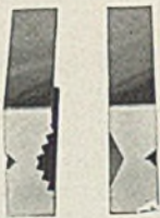
Standard vise jaws which are reversible for holding either round or square stock or hex head bolts.
