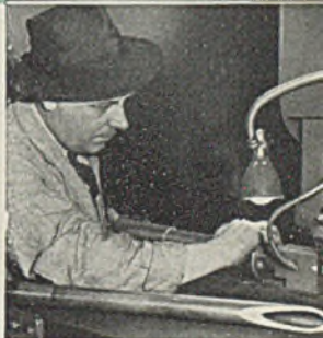
Steel alloy aircraft tubing cutoff production for airplane motor mounting frame work. New war-time job for this firm.
