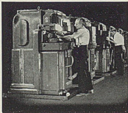
A battery of "Michigan" rotaries finishing gears in the plant of one aero engine producer.
