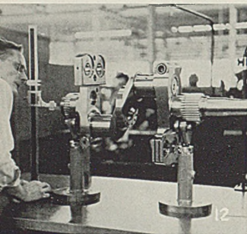
Fig. 10—In this Illinois gear checker, completed spline is being inspected after hobbing and grinding. Profile of tooth involute, being checked here, is held to 0.0002-inch
