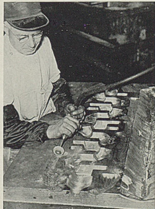
Fig. 5—Cavities are finished by hand. Here a die maker is working on a crankshaft die—highly specialized work that requires great skill
