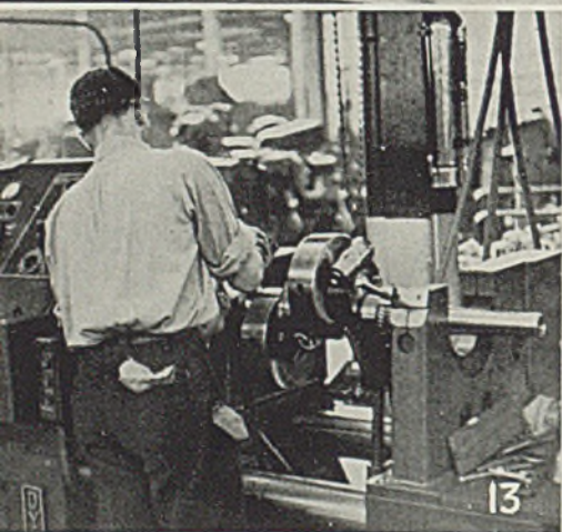
Fig. 15—Final inspection and touch-up of the finished shaft. Counterweights are not yet in place. Note highly finished main bearings
