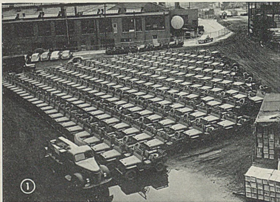
Fig. 5—Even the packing and crating department moves on an assembly line system. Wheels and windshields are removed and carefully packed before shipping. NEA photos
