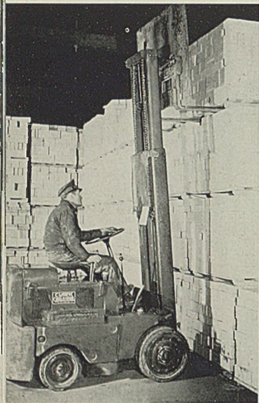
Fig. 4—Pallet loads are easily tiered four-high in the brick house as shown here. High tiering greatly increases capacity of the brick house by using "air" space
