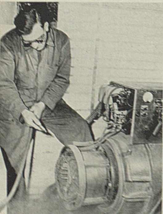
Fig. 5. (Right)—Card records on every welding machine in the plant will save time and money. Recordings made after inspection and service indicate any machine requiring excessive expense, the cause then can be corrected before an emergency occurs
