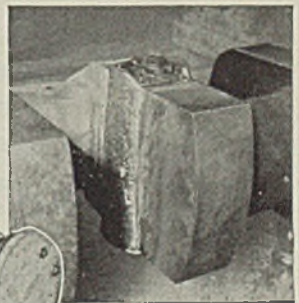
Close-up of Thermit weld, which has the strength and soundness of forged steel.
