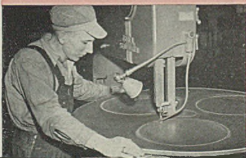
Cutting openings in 12 gauge 48" steel tank covers.
