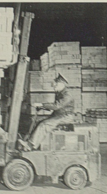
Fig. 3—Bricks, still loaded on their pallets, are placed on intra-plant flat cars for transfer to the furnaces. One operator, or at the most two, easily handle these unloading, storing and re-loading operations
