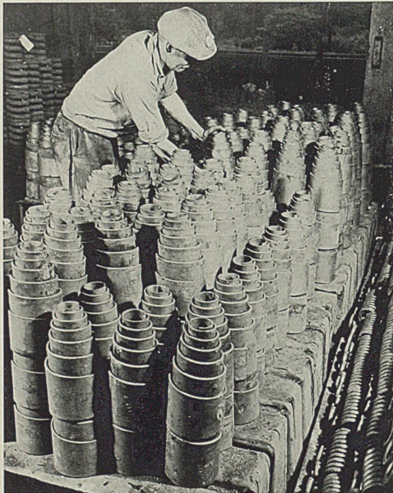
VOLUTE SPRINGS for light and medium tanks, made in American Locomotive Co.'s Chicago Heights, Ill., plant. With the exception of the spring shop the plant was closed down just ten years ago, recently reopened for manufacture of railroad supplies and war materiel
