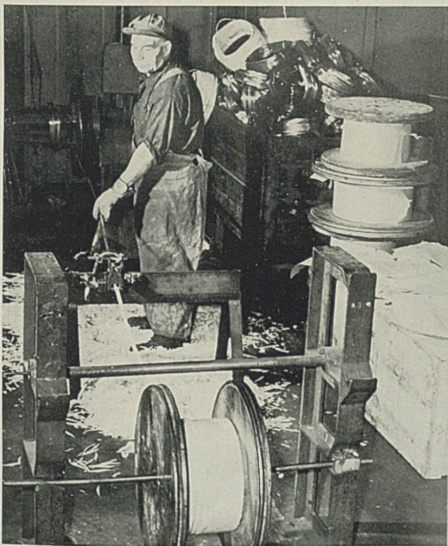
IN RECLAIMING wire in the salvage department of an eastern General Electric plant, even paper insulation is saved through the above operation which "skins" the paper covering from the wire. Paper thus salvaged is disposed of as high-grade paper scrap
