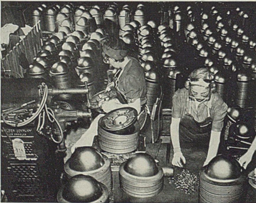
SPOTWELDING headband loops to the inside surface of steel helmets for use by civilian defense workers. Thousands are being manufactured for air raid wardens, police, firemen and Red Cross volunteers who form the "home front". Wide World
