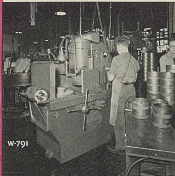
Grinding compressor heads on the No. 11 Blanchard Grinder
