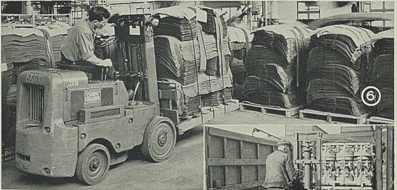
Fig. 6—Rubber mats can also cause handling difficulties. One way to solve them is to steel strap the mats on double-faced pallets as shown here. In this way, some 250 are handled by the fork truck as a single package
