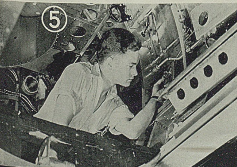
Fig. 5—Inspector employs special gage to measure the tension of control cables which must be adjusted to a specified value
