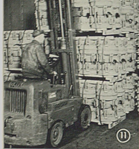
Fig. 11—Large volume of odd-shaped parts such as these castings are readily stored in a small area when unit packaging methods are used. Fork trucks can tier the packages to the ceiling, limited only by condition of the floors over which they must travel
