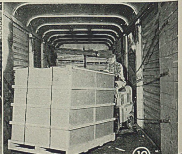
Fig. 9— Note how unit loads of axle castings are stacked to within a few inches of the roof of the storage area shown back of this fork truck handling a unit package of completed axle assemblies. Fig. 10—Unit packages are easily designed to utilize freight car space effectively. And the unit packages are effectively braced in the car by steel straps, yet can be quickly cut for speedy removal as shown here
