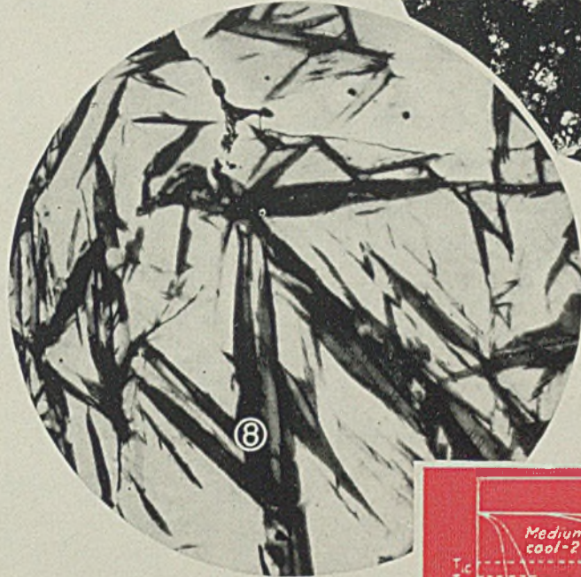
Fig. 8—Martensite at 1125 diameters. Note boundaries of original austenitic grains. Quenching rates in excess of critical produce this structure, sharply distinguishable from pearlitic structure produced by quenching rates below critical. Martensite consists of highly supersaturated, strained ferrite in which precipitation of carbides probably has not occurred to any great extent. Steel shown is high alloy type, heated to 2300 degrees Fahr. and quenched in oil. Some intergranular oxidation due to overheating may be observed. Bausch & Lomb photo
