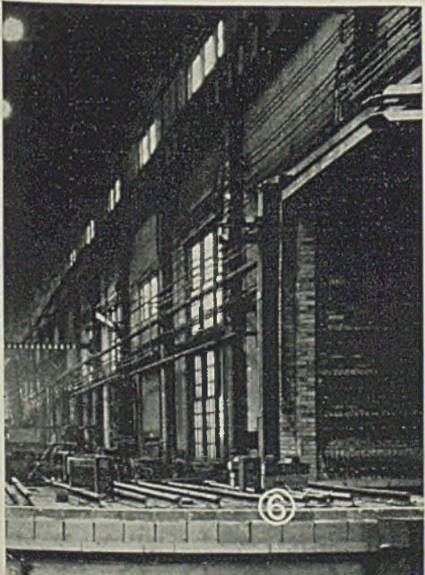
Fig. 10—Vertical cylindrical furnaces, electrically heated, are 30 inches diameter and 60 inches long inside, have transfer hoods and protective atmosphere for hardening and drawing
