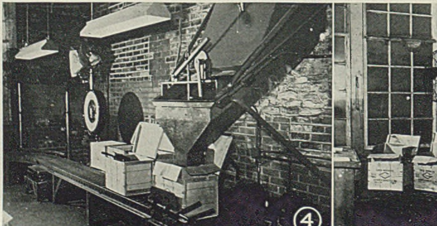
Fig. 5—Now box is moved down the conveyor line to a point where a built-in scale precisely measures the weight. Here a workman with a hand scoop removes or adds washers to produce the exact weight desired in the package
