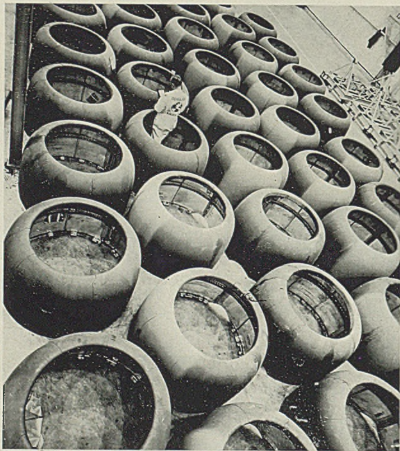
Aluminum alloy cowling such as these are used to cool, streamline and protect the powerful engines of Douglas transport airplanes. The units seen here in a sub-assembly department of a Douglas Aircraft Co. plant will enclose engines having a total of more than 50,000 horsepower
