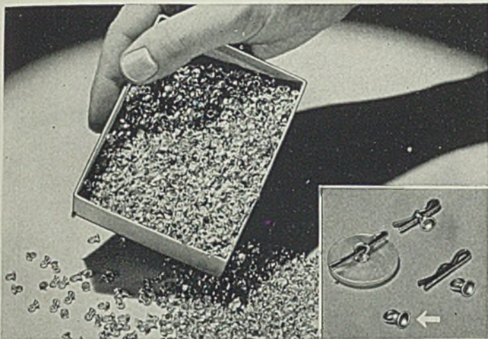
Shank shown in inset approximately \frac{1}{2} actual size—4,100 castings to the pound.
