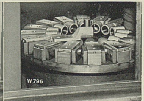
Grinding flat side of lugs
