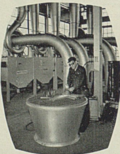
Grinding dust is pulled thru grills at the grinding stations and conveyed thru ducts in pipe trenches to the Roto-Clone Precipitators.
