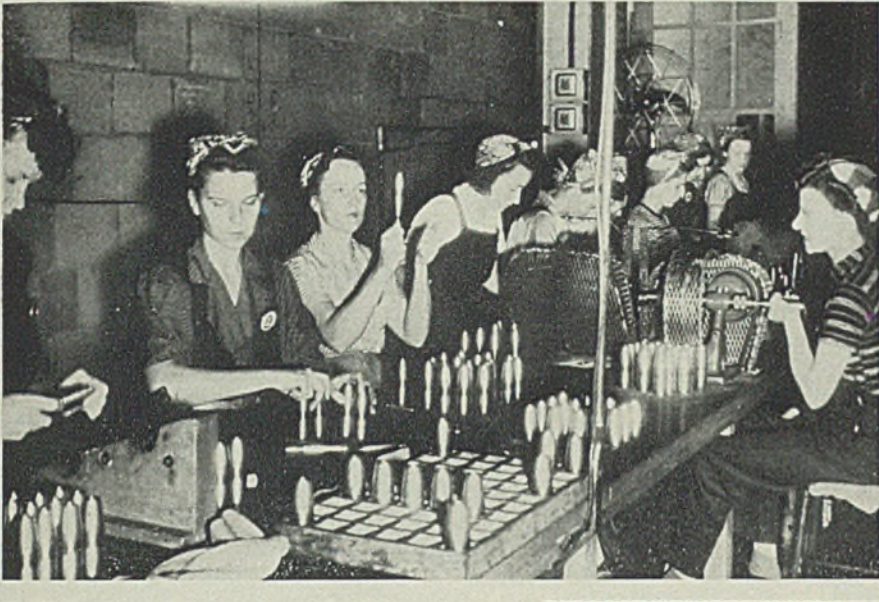
Skillfully trained women gradually are replacing the men employes in the small shell department of Oil Well Supply Co., United States Steel Corp. subsidiary, in Oil City Pa. Training program was undertaken by the company months ago, and the girls now are gaging, threading noses, and inspecting the high explosive projectiles
