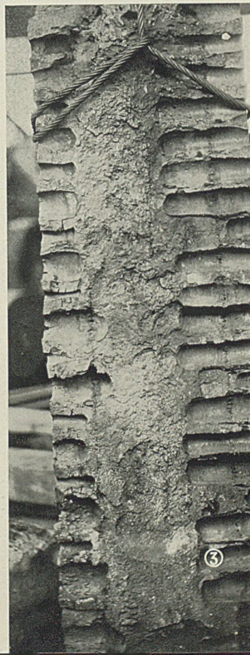
Fig. 3—Low carbon rimmed steel made with an iron charge of 69 per cent
