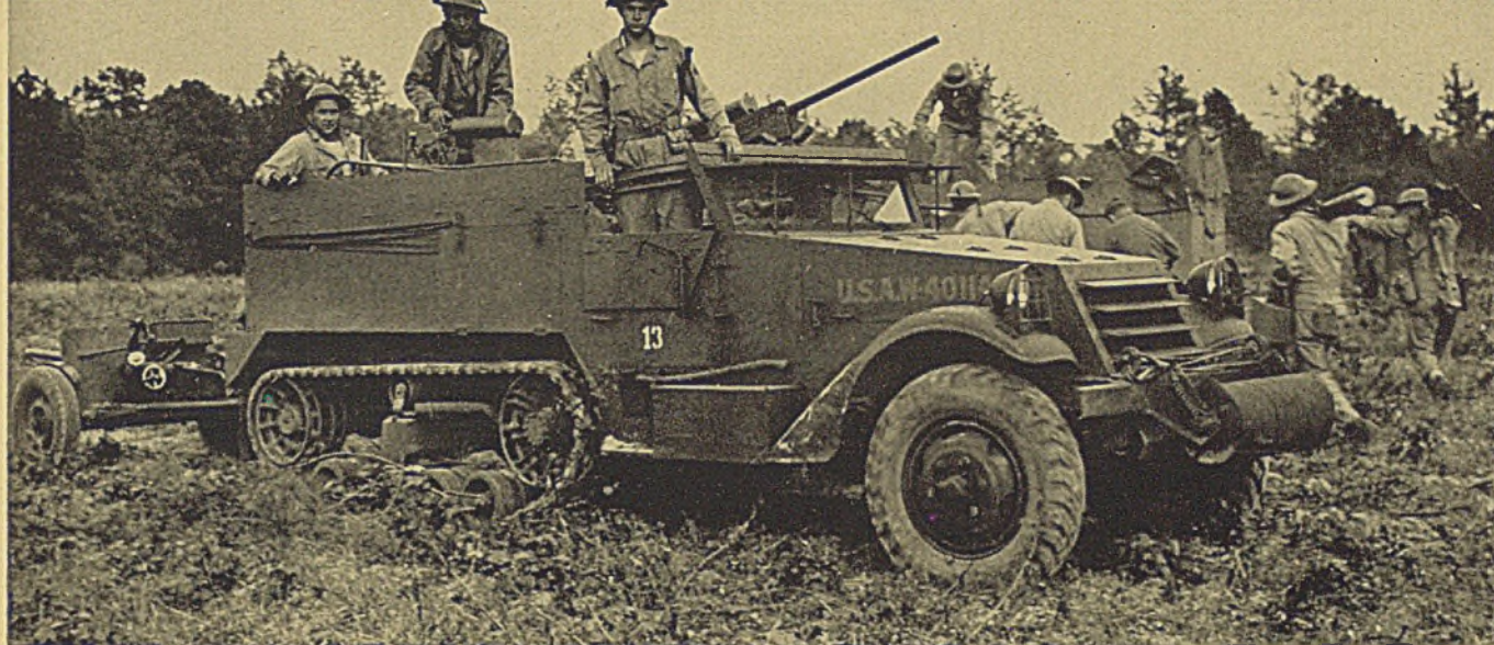
Fig. 6—Light rolled armor plate forms body of this half-trac scout car seen here towing a 37-millimeter gun
