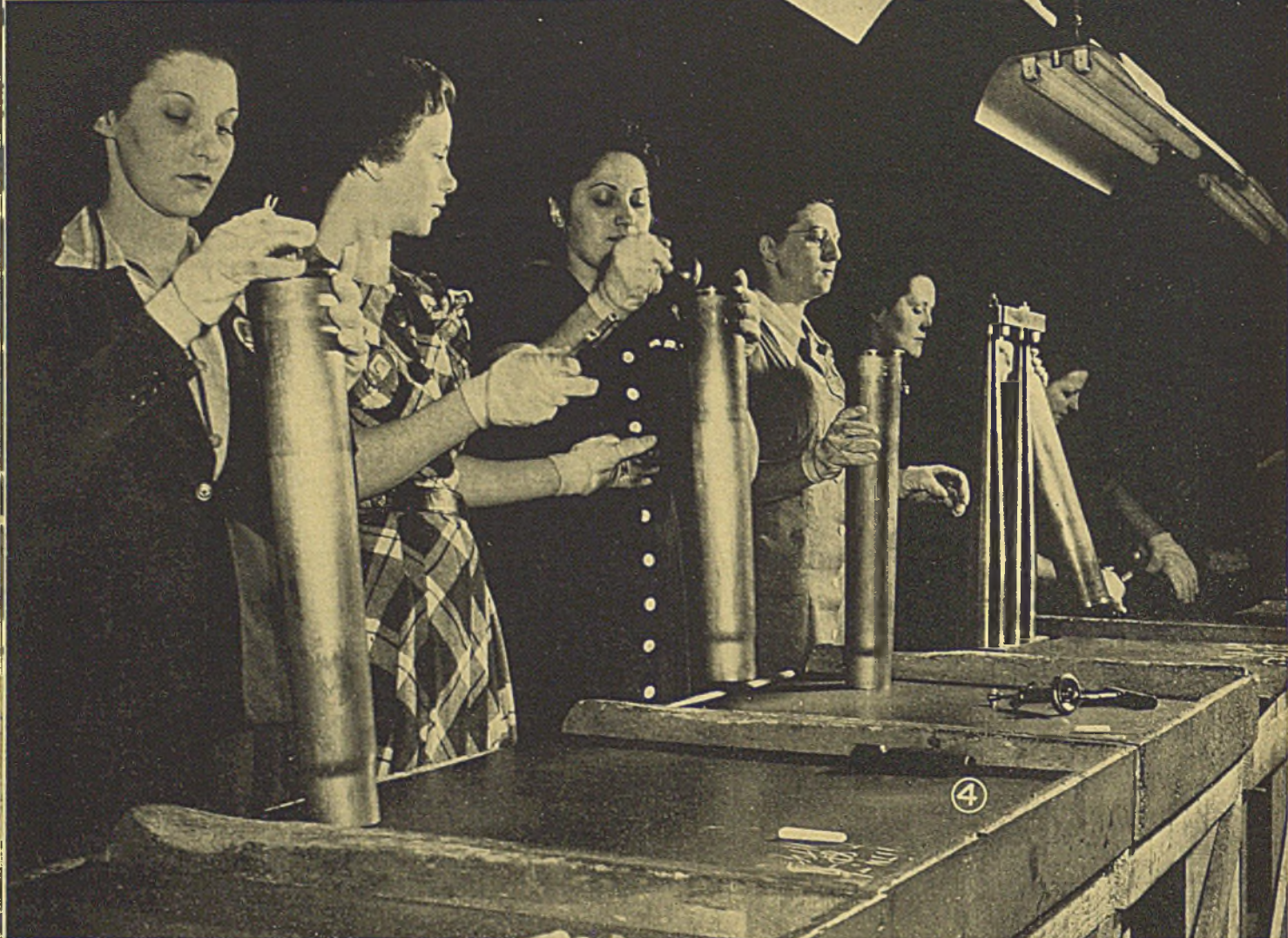
Fig. 4—Cartridge cases for 3-inch anti-aircraft guns. Copper of which we are short, constitutes 70 per cent of the billions of brass cartridge cases we need. Intensive research and experiment have produced a successful steel case, adequately proofed against chemical interaction with the powder charge
