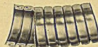
American Interlocked — wound of strip metal, joints packed; the toughest type of extremely flexible metal hose.
