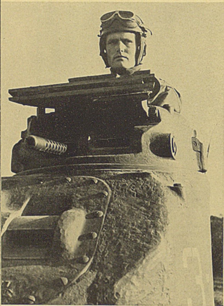
Fig. 7—Closeup of M-3 tank showing portions of cast armor forming the hull and turret. Certain sections such as gun mounts and shields are bolted in place for quick replacement in the field. Figs. 6, 7 and 8 from United States Signal Corps
