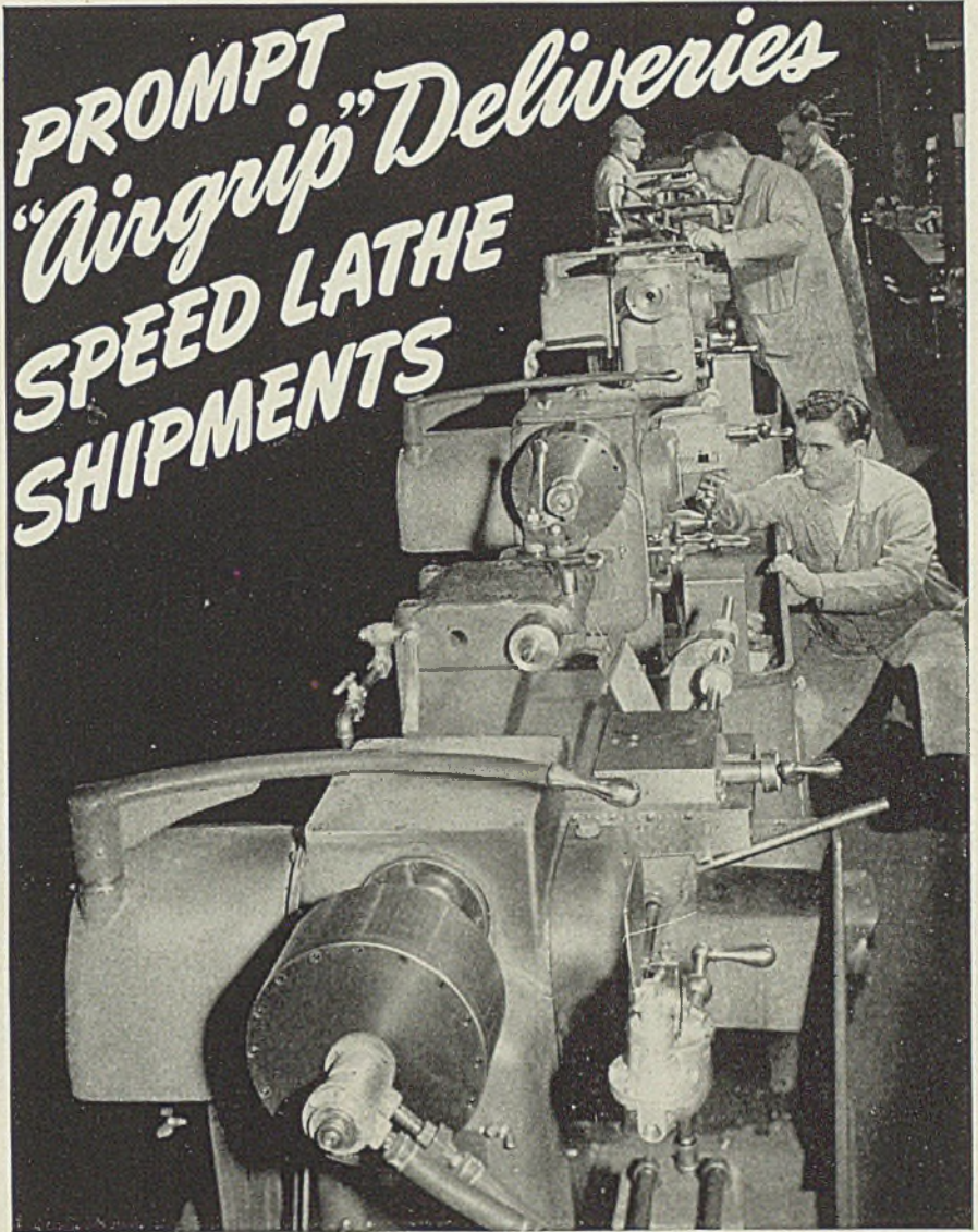
"Airgrip" cylinders being installed on Lipe Carbo lathes at the plant of Lipe-Rollway Corp.
