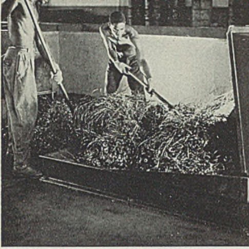
Chip-handling system at Wright Aeronautical gathers tons of scrap without hindering operations, p. 84
