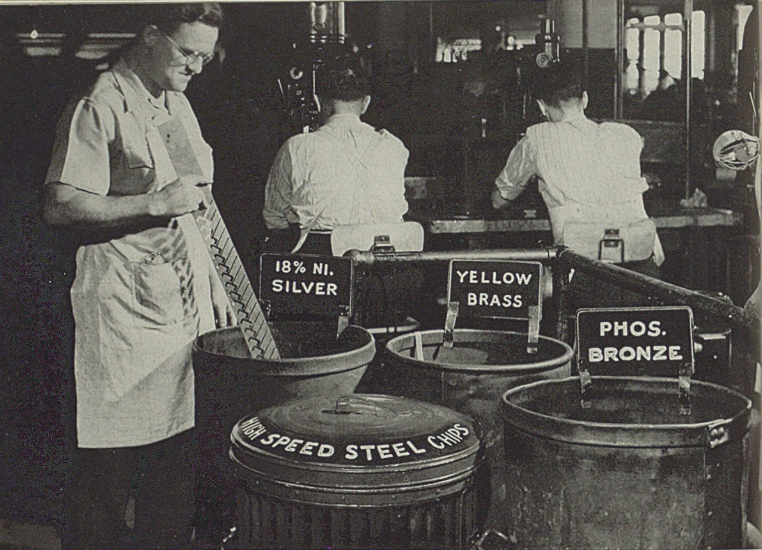
Proper scrap metal segregation avoids loss of valuable alloys.
