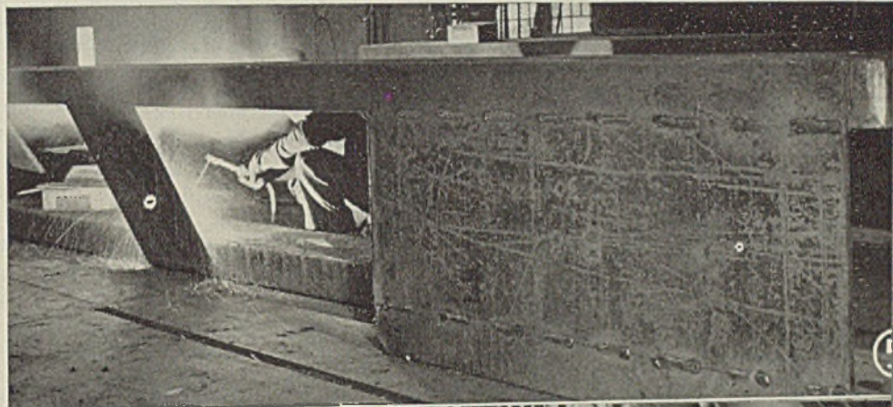
Fig. 3—Construction time for this 18-foot lead pan was short, for it consists of sections of standard plate thicknesses and rolled angles, flame cut and arc welded. Skip welding is important in such structures as this
