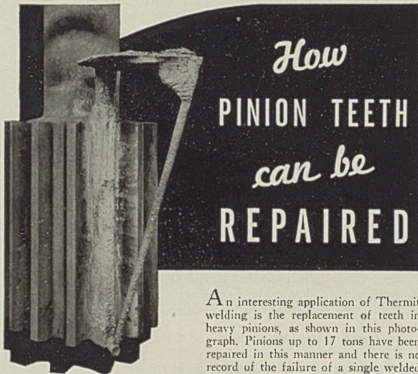
Pinion Repaired by Thermit Welding. Risers and Gates Not Yet Removed.
