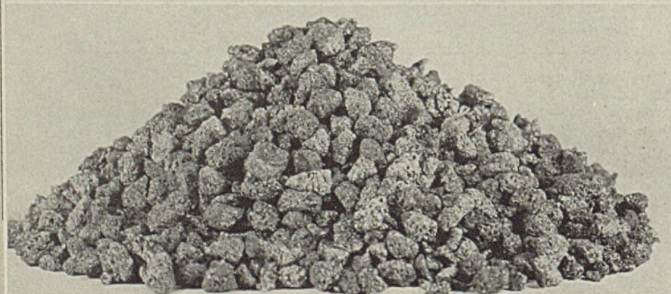
Fig. 1—(Upper left)—Nonburning carburizer before crushing and screening, showing inner cell impregnation of energizer
