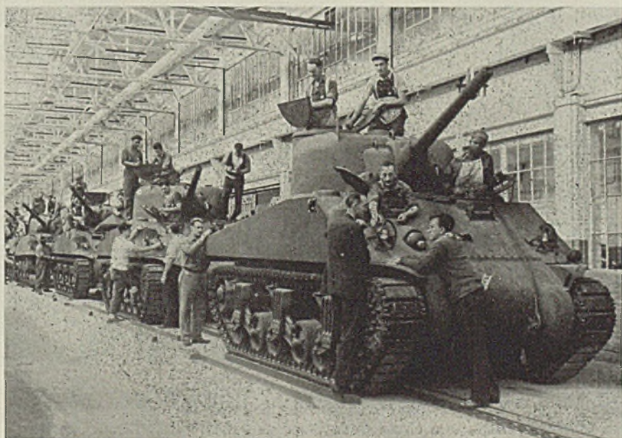
First picture released of assembly line on which 32-ton M-4 medium tanks are being built by Ford Motor Co., Detroit. Ford engineers have pioneered a number of innovations in design and construction
