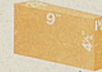
9" No. 2 Wedge 2'3" Inside Diameter, 3'9" Outside Diameter 57 Brick to the Circle
