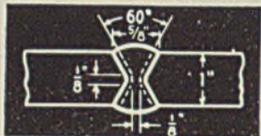
2. Partially grooved 60° Double-V Butt Joint
