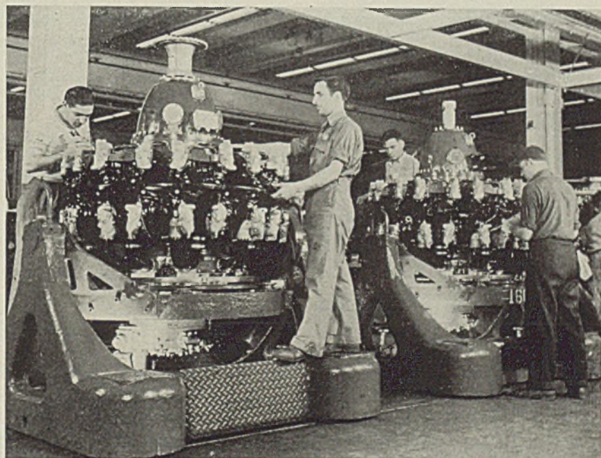
EXPERIENCE gained by Ford engineers in mass production of automobiles has been called into play in the volume manufacture of Pratt & Whitney aircraft engines, shown above on the assembly line where each workman performs a specific task. NEA photo
