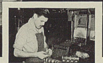
The operator assembles the parts and places them on the furnace conveyors.
