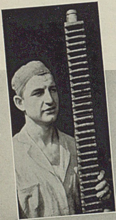
Fig. 1. (Left)—This gun broach cost $980 but became just so much scrap when all teeth were worn down 0.005-inch. It would have taken months to replace it, but Suttonizing enabled the unit to be put back into production in a few hours. New metal was welded on the teeth as shown
