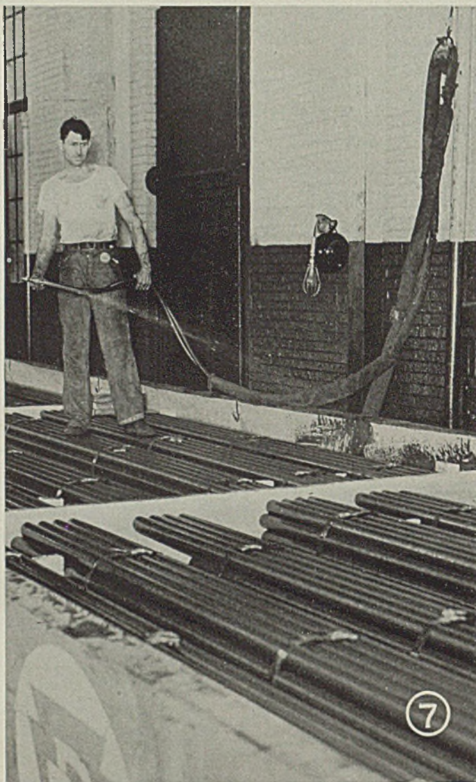
Fig. 7—Regulation spray gun equipment on 25-foot lengths of hose is used for spraying finished steel with slushing oil for protection during shipment. Oil and air outlets have quick-coupling connectors, consisting of socket and plug
