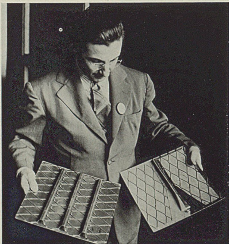
Peter Altman, director of the manufacturing research department of Vultee Aircraft Inc., inspects two different sample panels of the composite expanded steel sheet
