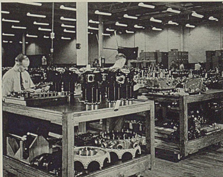
Two of these wheeled tables hold the 8000 parts making up one Wright engine as it is torn down for inspection after the "green" test run. Note forged steel crankcase sections on lower shelf of table at left
