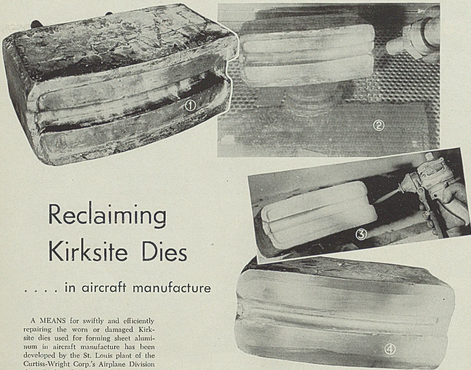
Fig. 1—Worn Kirksite die generally considered as being beyond repair. Note die has already been marked for scrap
