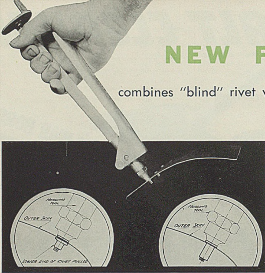
Fig. 1—Hand tool for setting up Rivnuts. Inserts show, right, Rivnut inserted from the outside on a tool and ready for heading; left, lower end of Rivnut pulled up by tool to form head on inside of work
