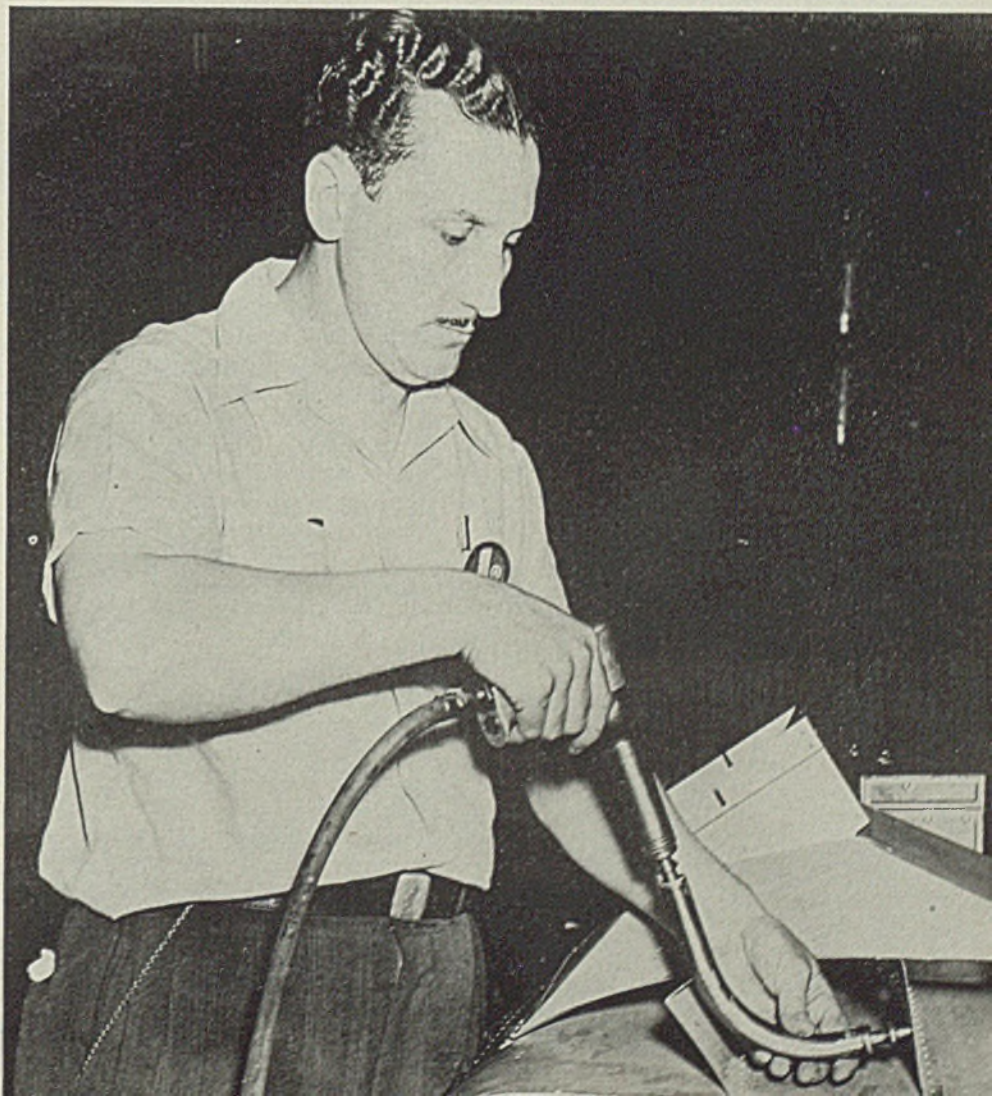
Fig. 4—(Below)—Jim Porter using the riveting hammer with bent peen devised by him for use in cramped spaces. This has speeded production by making what had formerly been a long irritating job a quick and simple one
