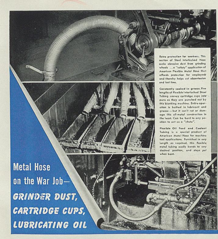
Using virtually any workable metal, we can furnish flexible hose or tubing for anything from a simple spout to a high pressure hydraulic line (American Seamless) that can be flexed millions of times without breaking.
