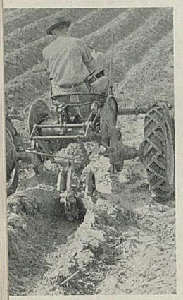
Farmall-A tractor, shown above, is pulling a one-row middle buster, an implement widely used in the South and Southwest. The tractor will cover 11 acres a day in middle busting operations
