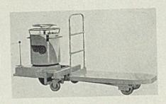
nal expanding brakes on the two load wheels. Operator's platform of this newer unit is 4 inches wider than those of previous models.
