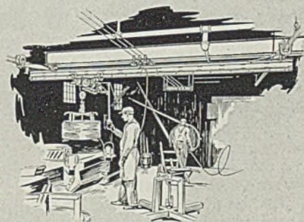
Stripping crane speeds up removal of wire coils.
