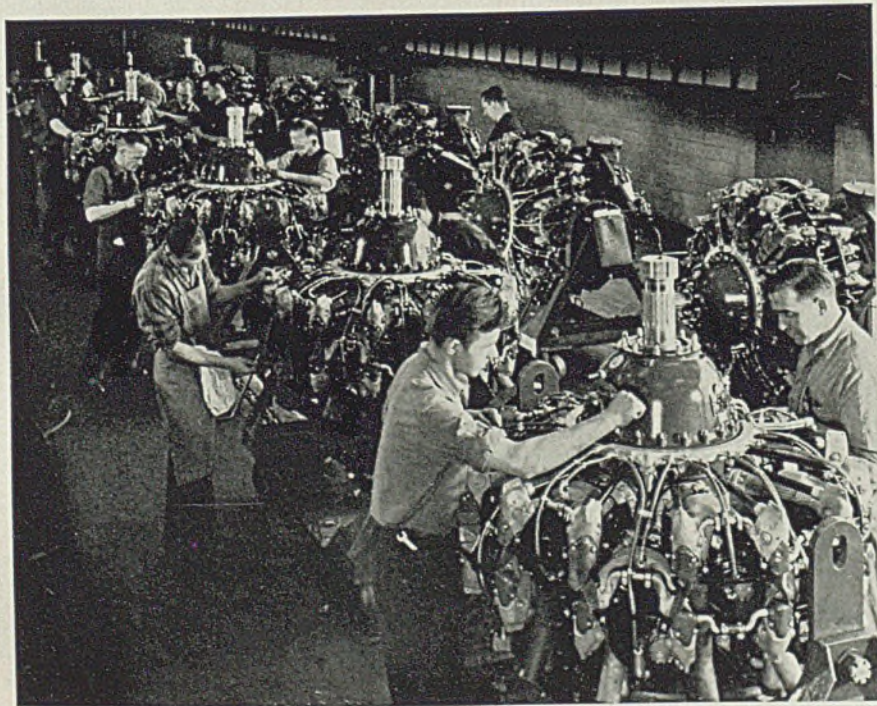
One section of aircraft engine assembly line at new Buffalo plant. Engines are mounted on special dollies moved along by floor chain. Fixture permits turning engine to any angle for ease of operators
