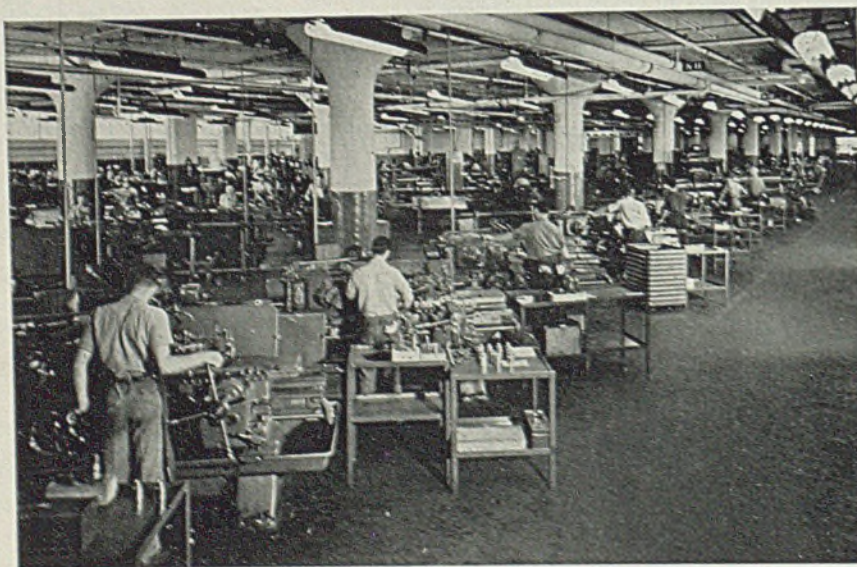
Former motor car assembly plant now re-equipped for small parts manufacture this area housing batteries of turret lathes. Provocative question is: What happens to all this beautiful new Defense Plant Corp. machinery when reconversion to peacetime production becomes practicable?
