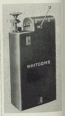
handwheel until the work is held securely between a rising V-block and a lowering button. When tight, the work is in line with the center line of the spindle and the hand lever advances the center drill to the work. The operator moves only the handwheel and the lever, it is said.
