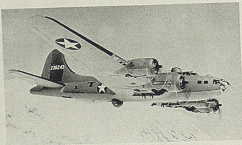
LARGER TALONS: The new external bomb racks give America's war eagles larger talons for heavier bomb loads. This recent photograph of a Boeing B-17-F Flying Fortress shows the forklike fingers of the two additional racks at the fuselage bottom near the wheels. The device permits much heavier bomb loads for limited-range operations
