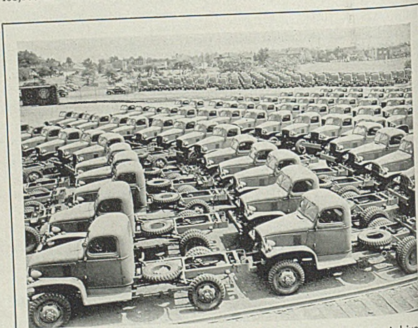
GOING "OVER": These Chevrolet military trucks, some four-wheel-drive and others two-wheel-drive units, are awaiting boxing for overseas transport at a seaboard export plant. To conserve shipping space the trucks will be torn down and boxed in compact weatherproof containers especially designed for the purpose
