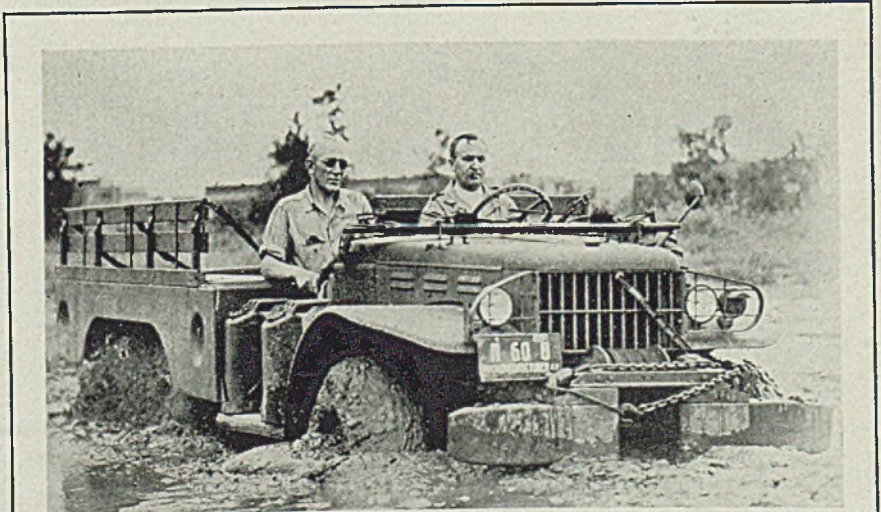
MUD TO MOUNTAINS: This new "low silhouette" 6 by 6 cargo and troop carrier truck is now being built in volume for the Army at the Dodge truck plant in Detroit. Accommodating 16 men with supplies, the truck will negotiate wheel-deep mud or water, climb a 62 per cent grade with full load, or—with tires deflated to 8 pounds—operate speedily through desert sands. Low overall height, combined with increased road clearance, improves the vehicle's tactical value for use in combat areas
