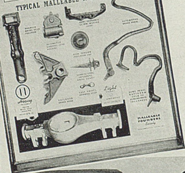
Figs. 8 and 9—Malleable iron in motor vehicle gun mount. Fig. 10—Eyebolt lifting lugs. Battered one at left shows resistance to impact. Fig. 11—Display of malleable applications prepared by Malleable Founders' Society. Fig. 12—Pearlitic malleable rollers for tank track
