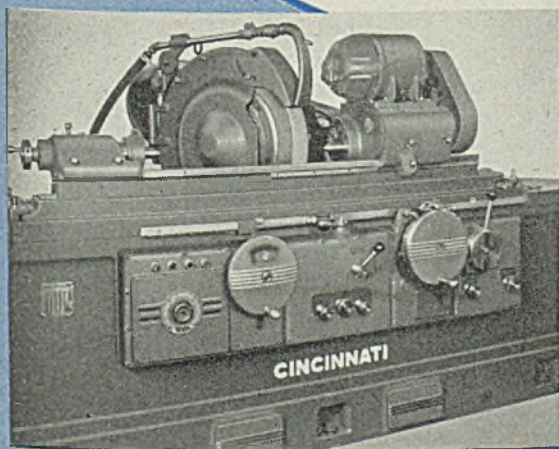
● Two close-up views of a CINCINNATI 10" Plain Hydraulic Grinder tailored to suit the job... wheel-head set at a 30^\circ angle; headstock and footstock interchanged; automatic infeed attachment.
