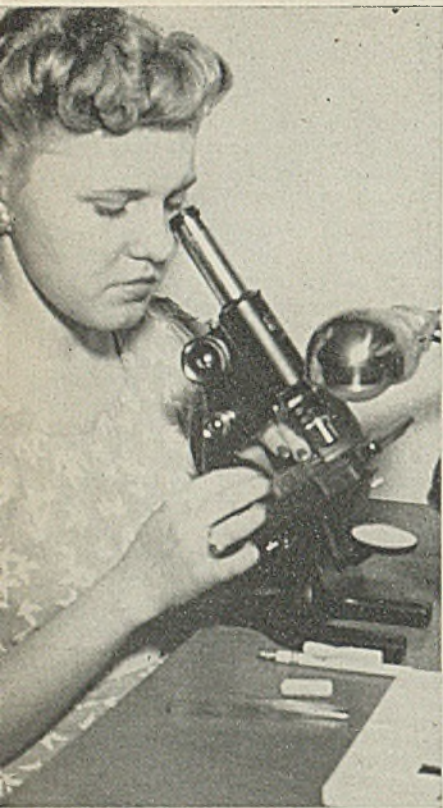
Fig. 5—Drill dimensions are checked against a scale on the eyepieces of the 200-power microscope. Rejections, even under 0.0001-inch tolerances, are unbelievably small
