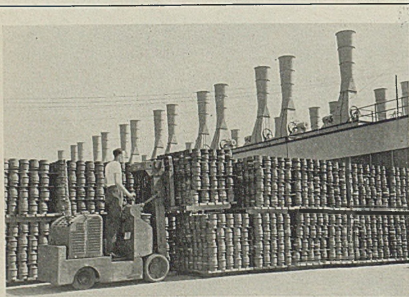
HANDLING AIRCRAFT FORGINGS: Gas-electric lift truck picks up a pallet of 160 alloy steel cylinder barrel forgings from yard storage at the Melrose Park, Ill., plant of Buick Motor Division, to move them into the machining department where each 30-pound forging loses about two-thirds of its weight before installation in a Pratt & Whitney 18-cylinder aircraft engine. In the background are some of the exhaust stacks from the engine test cells at the plant. Note blowers on each stack to provide forced draft, necessary since engines in cells drive generators and not propellers which would provide the desired air circulation
