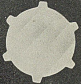
31 Rod with Six Lugs machined in Screw Machine
