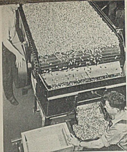
Billions of small steel cartridge cases, and each must pass 334 kinds of inspection. Page 126
