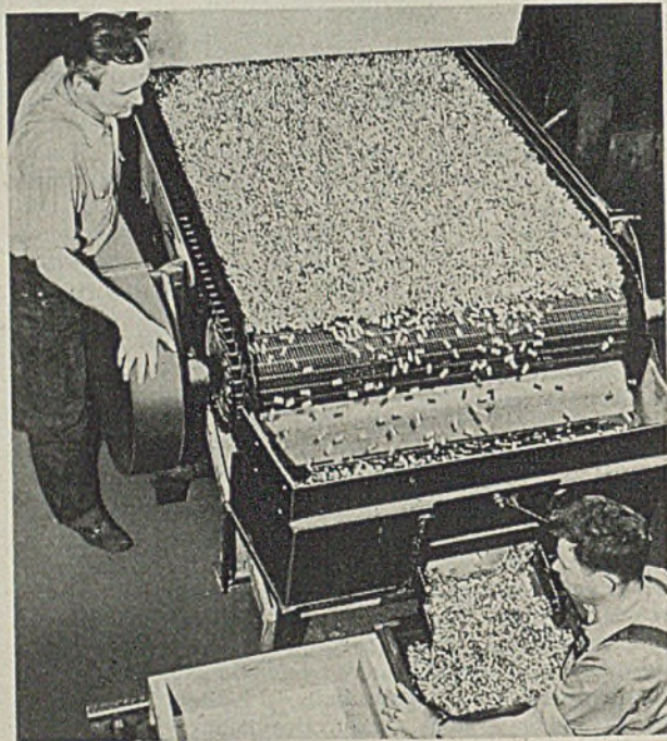
Fig. 1. (Above)—One of the 334 inspections given each round of ammunition. Here girls are gaging and inspecting steel cartridge cases, placing rejects in boxes labeled for such defects as scratches, dents, long case, short case, broken punch mark, poor identification, round heads, bad plating and laminated metal
