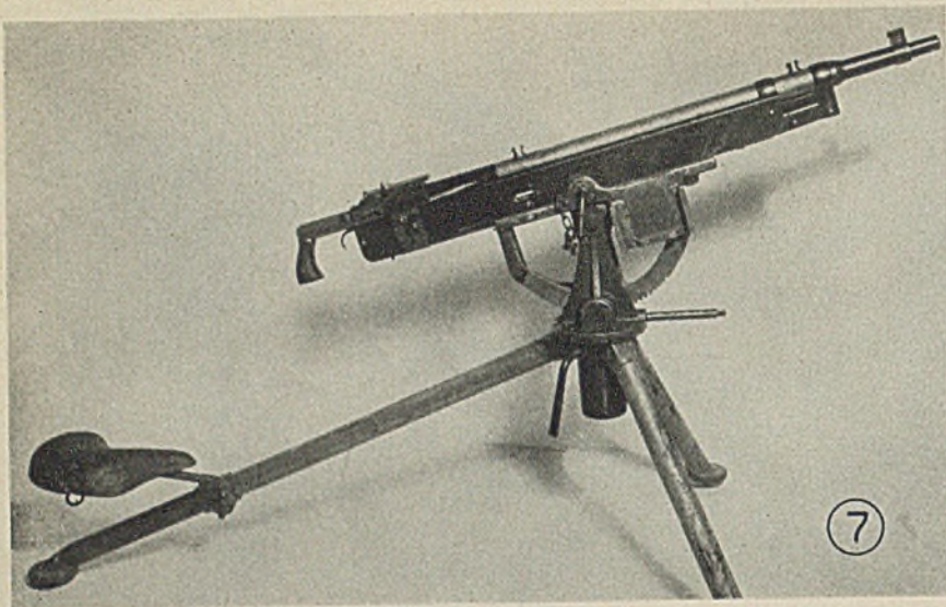
Fig. 7—Italian Colt heavy machine gun was made in the United States. It is a modified 1915 model
