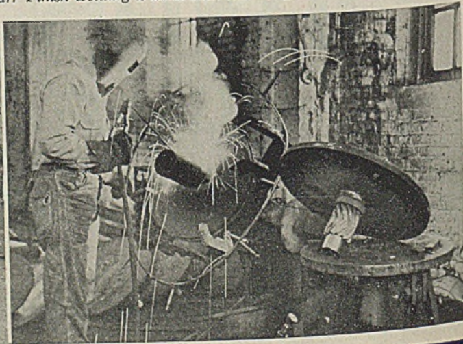
Fig. 5 (Right, below)—Parts such as this completely machined and heat-treated pinion gear must be protected from weld spatter during tackwelding and finish welding. Here setup fixture on which finished assembly sets provides enclosure for gear. Finish welding is done with tubular guard over gear as shown
