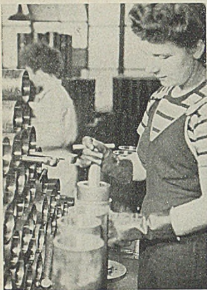
Fig. 11—Inspecting bore diameters and counterbore depth, operation 9, Table I
