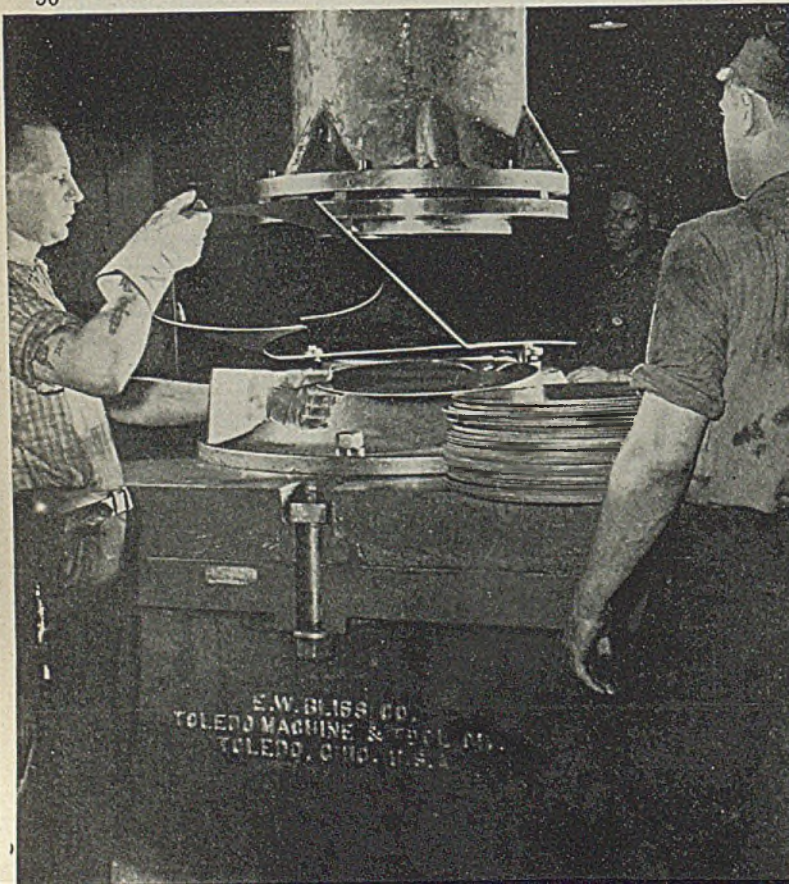
Fig. 2. (Right, below)—Forty per cent of total reduction is achieved in first cupping operation. Cups are ejected into a pit below the press, removed by conveyor and loaded on trucks for removal to the mechanical cleaning and annealing department. Cleaning and annealing follow every draw
