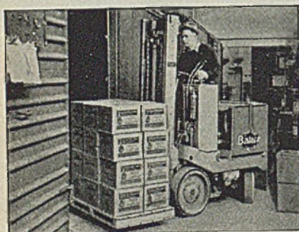
Box car or truck loading is speeded by handling pallet loads with fork truck.
