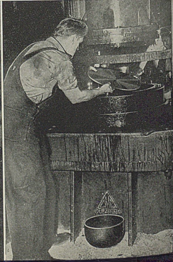
Fig. 2. (Right, below)—Forty per cent of total reduction is achieved in first cupping operation. Cups are ejected into a pit below the press, removed by conveyor and loaded on trucks for removal to the mechanical cleaning and annealing department. Cleaning and annealing follow every draw
